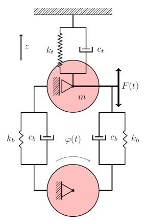
Analysis of the scheme allows to claim its number of degrees of freedom which is 1
